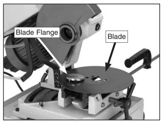
Figure 24. Blade removed.
